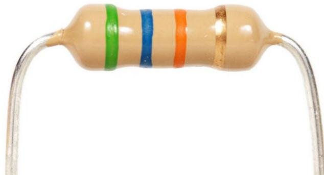
Gambar 5.1 Resistor 5600  $\Omega$
